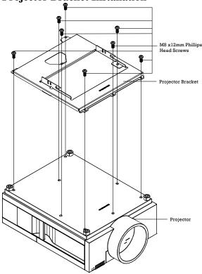
**Step 1**. Invert the projector and place it on a soft and flat surface. Remove any foot levelers that might possibly prevent the correct installation of the bracket.
